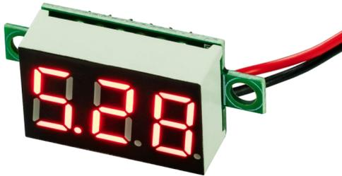
This small mini voltmeter for voltages from 3 to 30 V has a 3 digit 7-segment display (0.36 Inch). The measured value can be displayed with 1 or 2 decimal digits and is refreshed every 0.3 seconds. This measurement device is outstanding by its very low power consumption of less than 30 mA and can be mounted using the 2 mounting holes.
