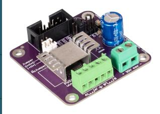
The PoStep25-256 is a high-performance, cost-effective stepping motor driver to implement intelligent stepping motor control – Smooth tune. The driver incorporates an advanced architecture and surface mount technology to archive an exceptional power density.
