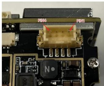
Figure. 5: LiDAR connector appearance
