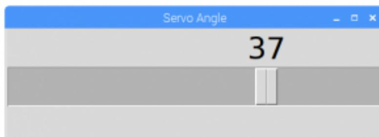
When you run the program, a window will open with a slider. Move the slider left and right and the servo should follow.
