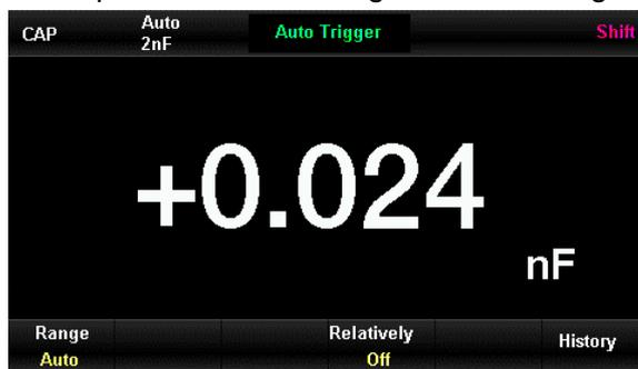
Figure 2-17 capacitance measuring interface
