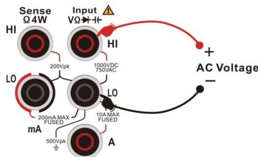
Figure 2-22 Connection of signal cycle measurement
