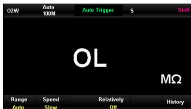
Figure 3-3 Reading of short-circuit test leads
