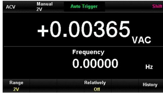
Figure 2-10 Interface of AC voltage and frequency measurement
