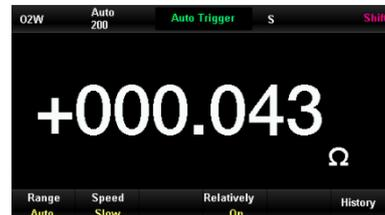
Figure 3-4 Reading after relative operation
